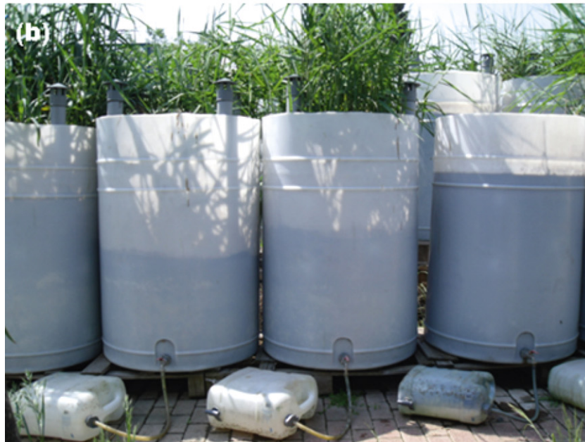
Fig. 1. (a) Schematic vertical section of the pilot-scale SDRB units [19,20] and (b) view of some pilot-scale units.
